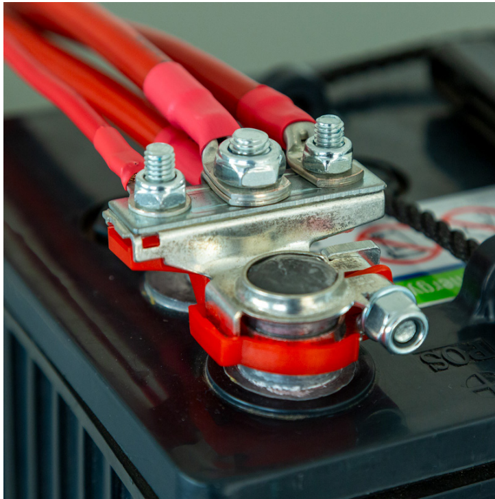
Figure 10 Battery cable connection (National Luna, 2021)
